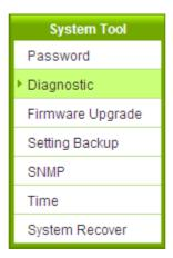
The device provides a simple online network diagnostic tool to help users troubleshoot network-related problems. This tool includes **DNS Name Lookup** (Domain Name Inquiry Test) and **Ping (Packet Delivery/Reception Test)**.
