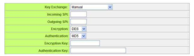
If there is any encryption mechanism, the encryption mechanism of these two VPN tunnels must be identical in order to create connection. And the transmission data must be encrypted with IPSec key, which is known as the encryption "key". The device provides the following two encrypted Key Managements. They are Manual and IKE automatic encryption mode- IKE with Preshared Key (automatic). By using the drop down menu, select the desired encryption mode as illustrated below.
